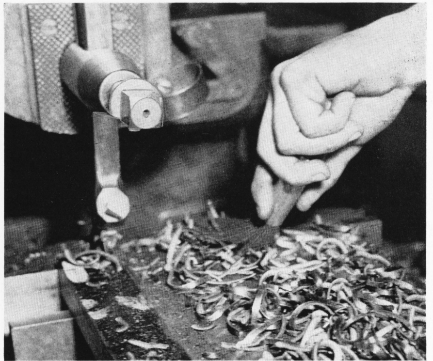
This picture shows a proper and safe method of clearing chips away from work. The operator is saving his hands from possible harm and dangerous infection.
